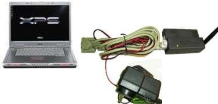
Setup example : Serial port connection to a PC
